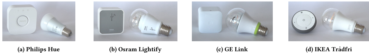
Figure 3: The four evaluated ZigBee-certified connected lighting systems.
